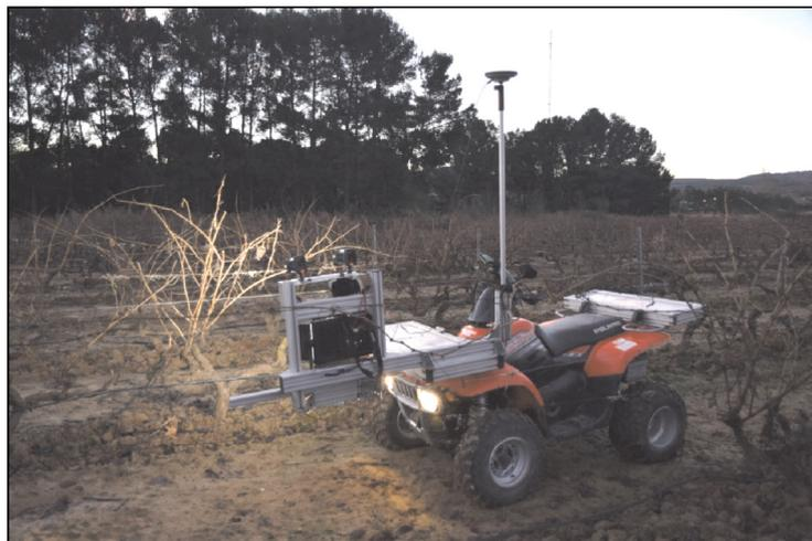
**FIGURE 1.** Mobile sensing platform: modified all-terrain vehicle (ATV) equipped with a digital RGB camera, automated triggering system, illumination on an adjustable structure and GNSS receiver for data georeferencing.
