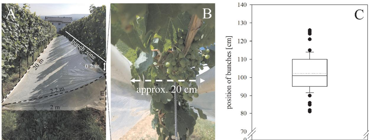
**FIGURE 1.** One side of the open heating system in the vineyard (A), close up of the opening of the open heating system in the middle of the bunch zone (B), bunch (n=67) height distribution above ground level (C).
