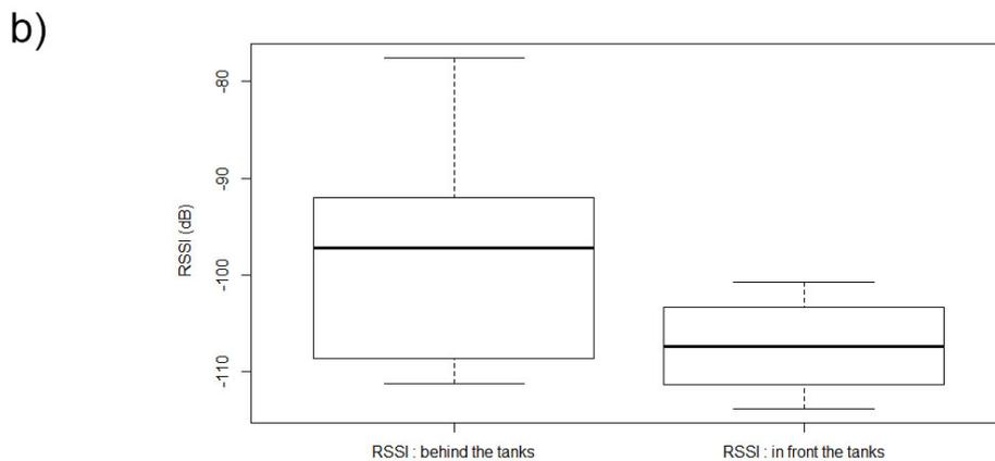
**FIGURE 7.** a) Signal reception quality as a function of the distance to the gateway antenna for end-devices behind or in front of the tanks, and b) comparison of RSSI variations with the sensor antenna outside and in the tanks by box plot.
