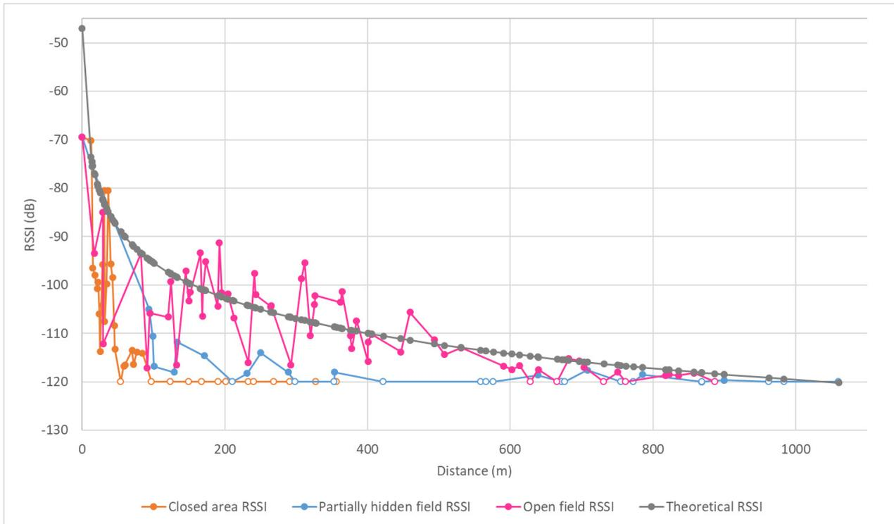
**FIGURE 4.** Signal reception quality as a function of the distance between the end-device and the gateway antenna for the three zones (closed area, partially hidden field, open field and theoretical RSSI).
