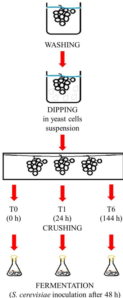
**FIGURE 1.** Schematic representation of the experimental procedure.
