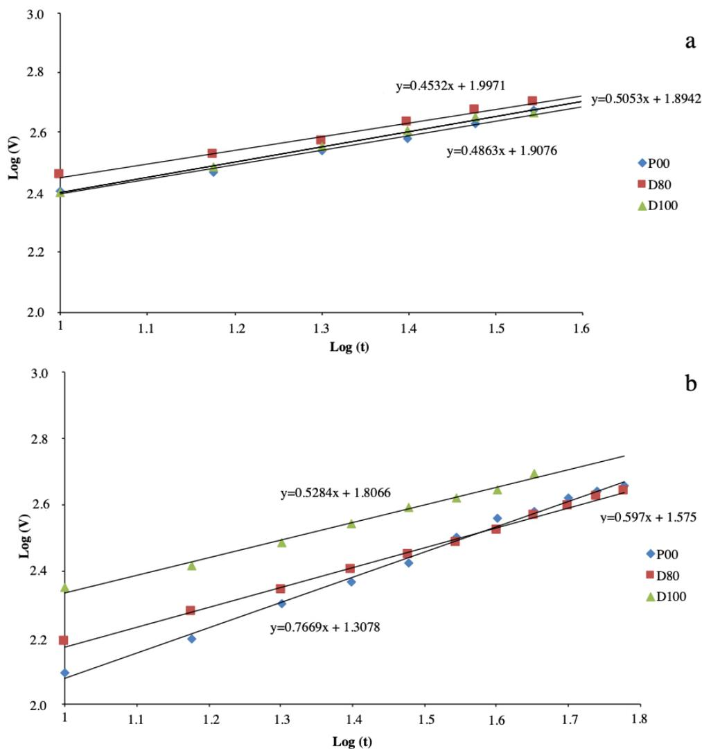
**FIGURE 4.** Evolution in logarithmic coordinates of the volume as a function of time of the filtration realised with Diatomyl® P00, Rilsan® D80 and Rilsan® D100 using the matrices 10.3 % DM (case a) 20.2 % DM (case b).
