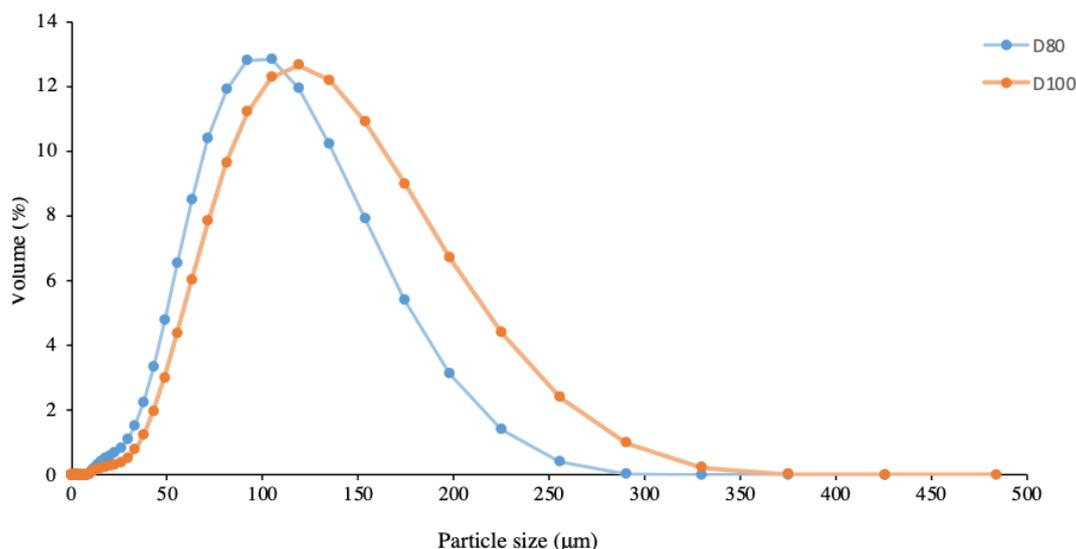
**FIGURE 2.** Particle size distribution for Rilsan® D80 and D100.
