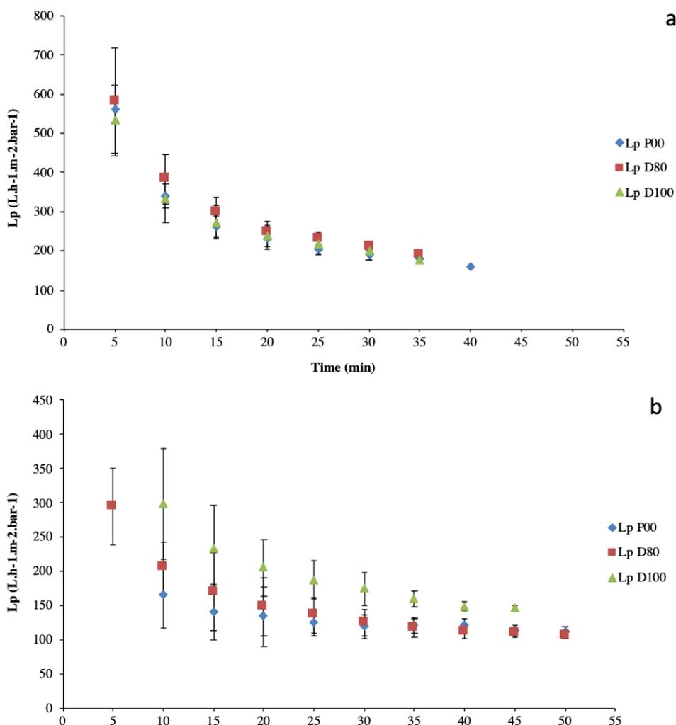
**FIGURE 3.** Evolution of the permeability (Lp) along the time for a solution at 10.8 % DM (case a) and 20.2 % DM (case b) for Diatomyl® P00, Rilsan® D80 and Rilsan® D100.
