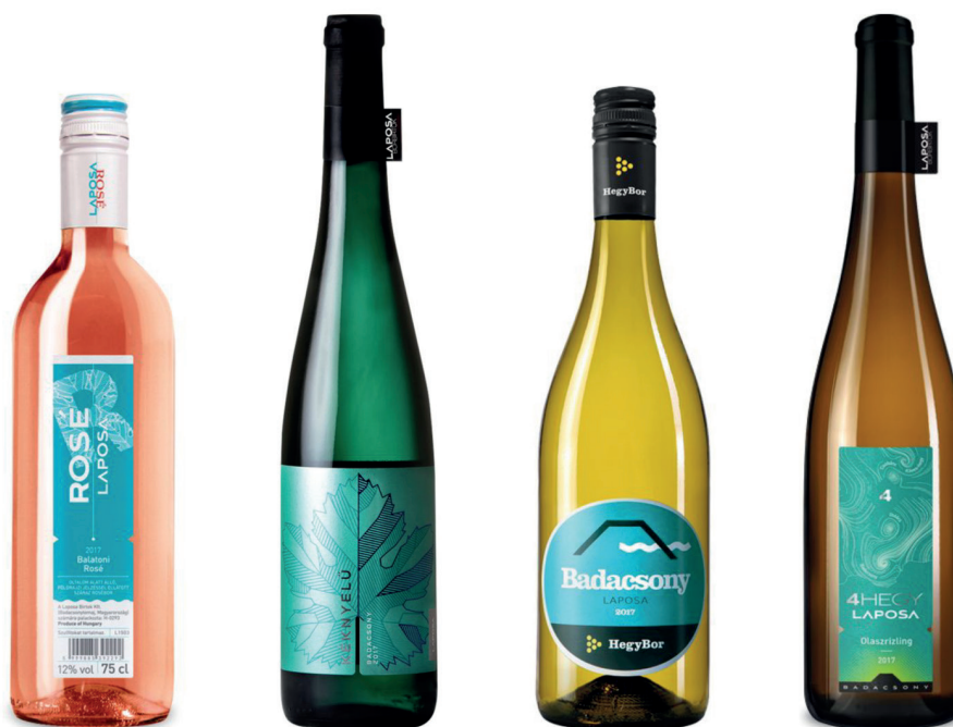
FIGURE 1. Wine bottles studied experimentally and modelled for light damage of white wine bottled in them. From left to right: clear (flint), bluish-green, light amber and dark amber bottle.
