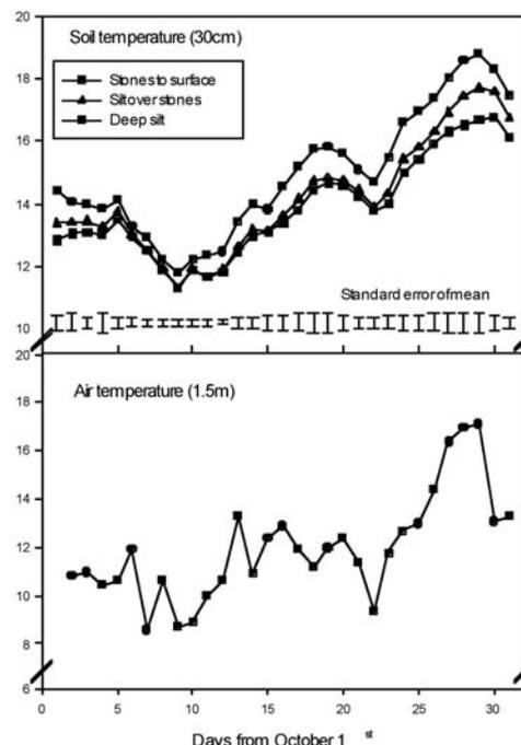
**Fig. 3 - Mean daily air temperature and the influence of depth to gravel on soil temperature at a depth of 30cm**
