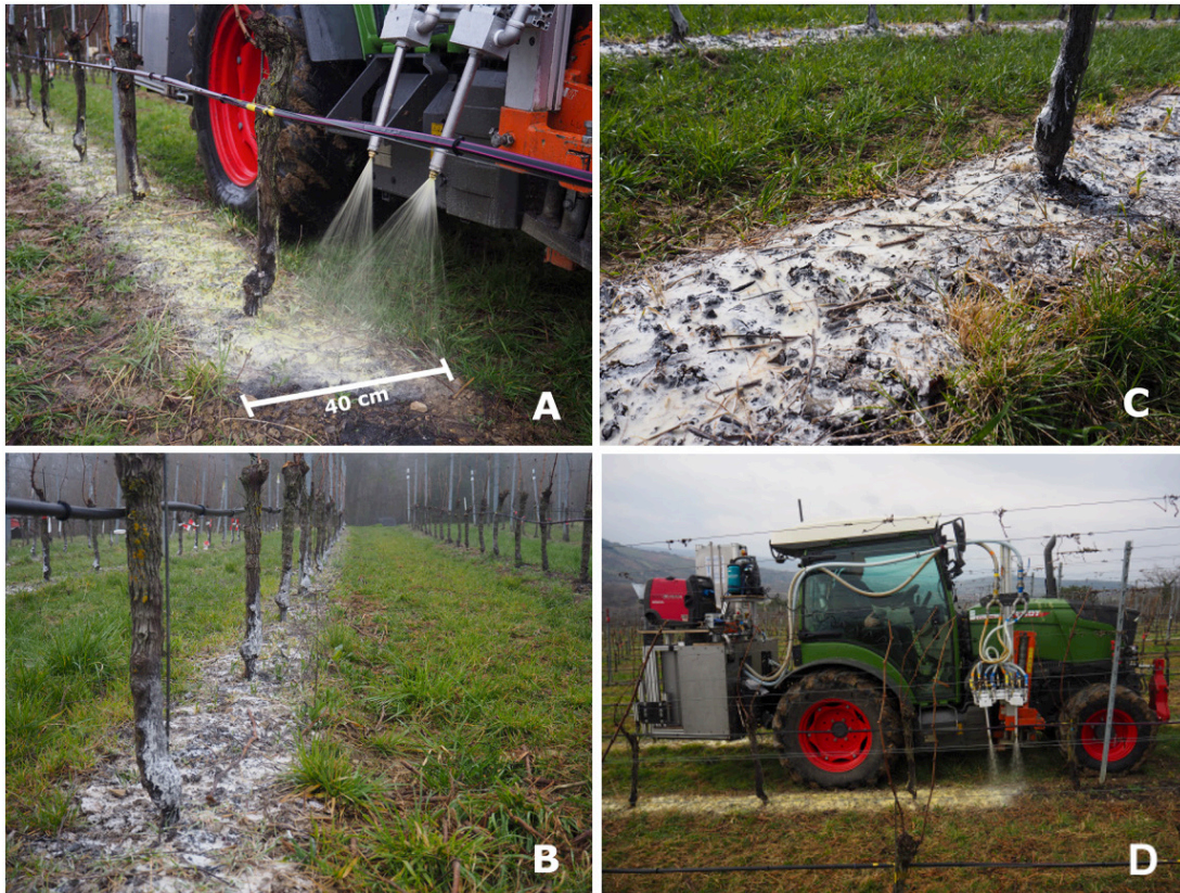
FIGURE 1. A) Application of the biodegradable-sprayable mulch in the field trial B in spring using the prototype developed by the project partner Technology and Support Centre (TFZ) Straubing; B) and C) The biodegradable-sprayable mulch forms a uniform, gel-like layer directly on the soil in the under-vine area, which later solidifies to ensure stability; B) 2.5 L m -2 of mulch was applied early in March 2024 (SM-2.5E) and C) 5.0 L m -2 of mulch was applied early in March 2024 (SM-5.0E); D) Application using the prototype tractor-mounted device.
