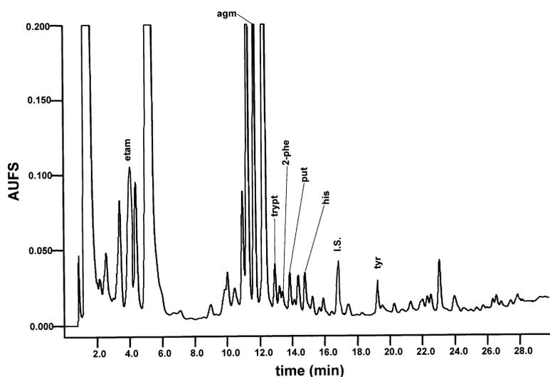
**Fig.2. Chromatographic separation of biogenic amines in a wine sample.**
